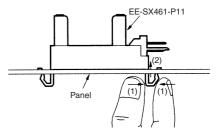
Pressed mounting holes are ideal for mounting the
