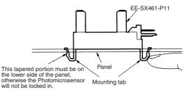
EE-SX461-P11 Photomicrosensor (Transmissive)
