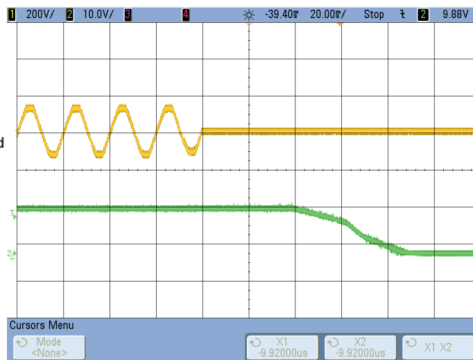
Figure 3 V1 hold up example at 250 W load with 90 VAC input (42 ms)
