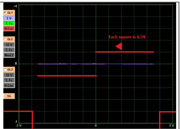
Figure 58: If the Test Voltage 2V, Each Square Represents 0,5V.
