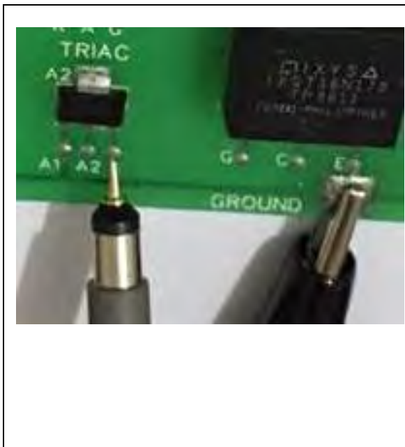
Figure 166: Channel1 Probe Used for Gate - Anode1 Measurement
