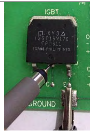
Figure 153: Channel1 Probe Used for Collector - Emitter Measurement
