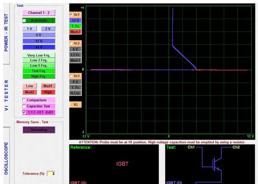
Figure 155: IGBT VI Graph, Equivalent Circuit Diagram
