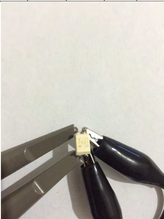
Figure 179: TLP521-1 Test Channel1 (Collector) - COM (Emitter)
