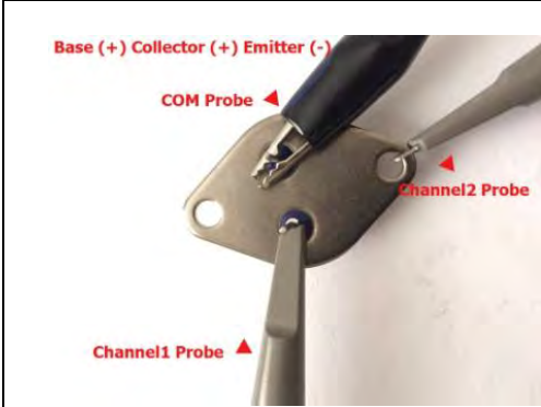
Figure 113: Channel1 (+), Channel2 (+), COM (-) Transistor Test
