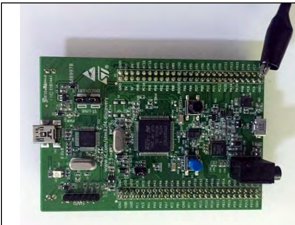
Figure 210: Connecting the Crocodile Probe Electronic Circuit Board Chassis (Step 1)
