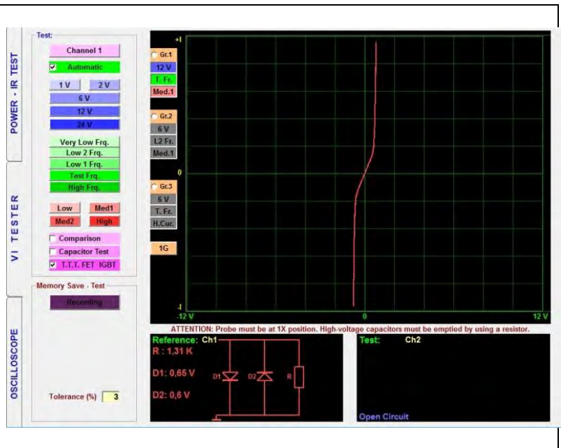
Figure 167: Gate (+) Anode1 (-) VI Graph
