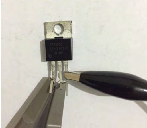
Figure 136: Channel1 (+), Channel2 (+), COM (-) Transistor Test
