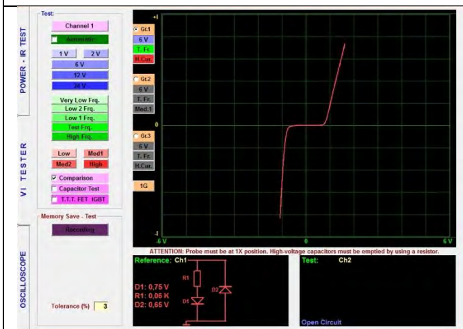
Figure 200: LM732 2MA In (-) VI Graph
