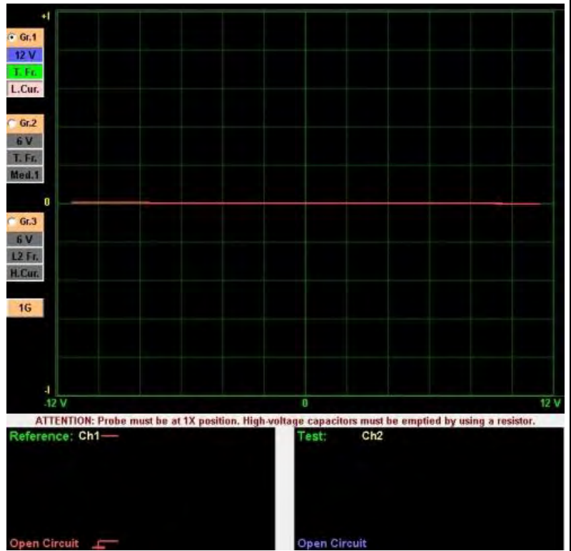
Figure 160: Gate (+) Anode (-) VI Graph
