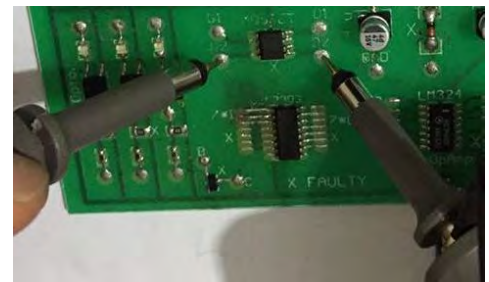
Figure 143: Sample of a Defective P Channel FET
