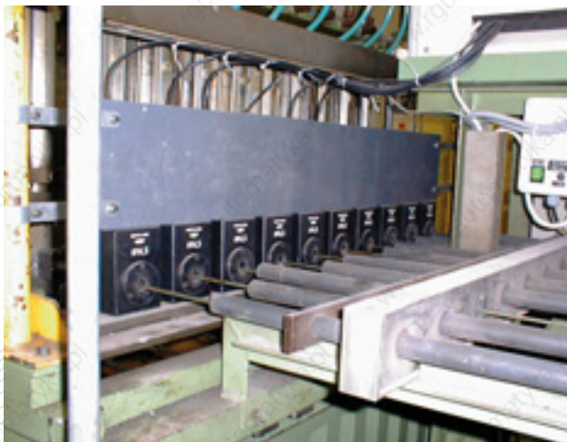
Multi-channel inspection with coils
