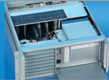
All kinds of drives can be installed behind the lockable front door.
