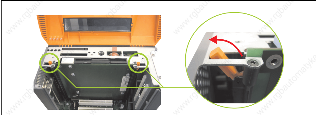
Figure 251: Release the slide-in slot releasing mechanisms
