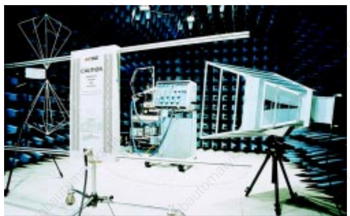
EMC Radiation testing
