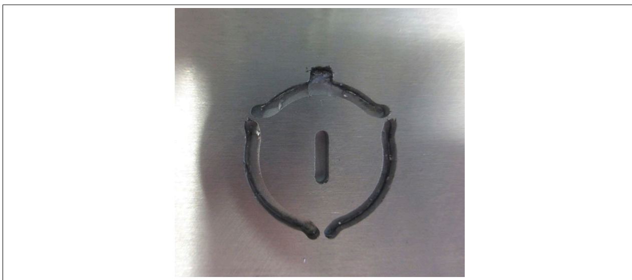
Figure 82: Cut the panel overlay along the cutout areas
