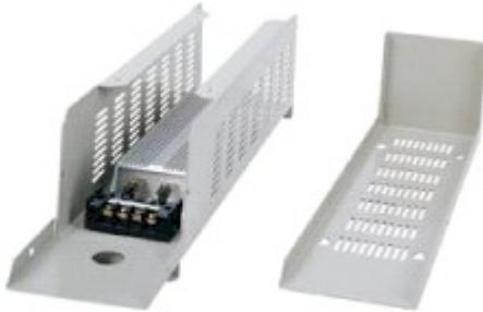
The RA series of power, metal clad, wire wound resistors are designed for use in power inverters. The basis for these models is an IRH or IRV resistor surrounded by a metal case, which conforms to international safety specifications. The steel case is powder coated and baked for durability.
