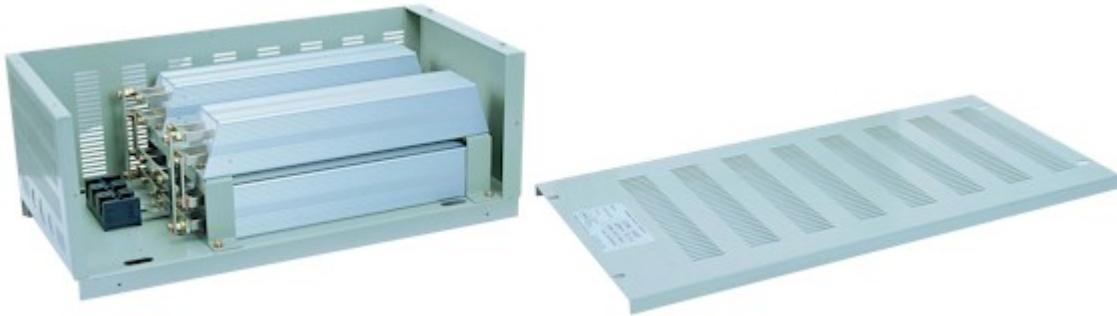
The HRA series of power, metal clad, wire wound resistors are designed for use in high power inverters. The basis for these models is an IRV resistors surrounded by a metal case, which conforms to international safety specifications. The steel case is powder coated and baked for durability.
