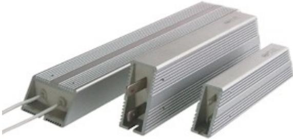
The IRV(V=vertical) & IRH(H=horizontal) models are our standard wire wound, metal clad resistors. The ULV and ULH models are UL approved versions of the IRV and IRH. These models have an extruded aluminum housing providing rugged and strong protection. Options include flying leads or tab terminals, inductive or non-inductive windings. The most common applications for these models are motor drives, braking and snubber applications and power sources for industrial equipment.
