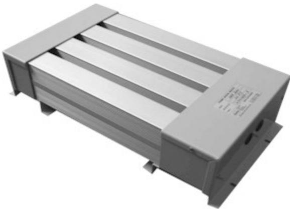
These economical and powerful components comprise two, three or four high power resistors housed in partial steel covers at each end. These rugged, powder coated covers ensure an excellent seal. The internal resistors use aluminum plates at each end instead of our standard cement molding. This innovation reduces construction time and reduces cost, at no reduction of performance. The major application of this exciting new model is highpower inverter braking units.
