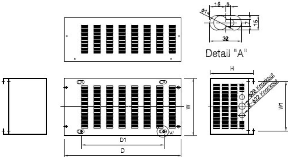
These models come with multiple conduit knockouts for easy wiring.
