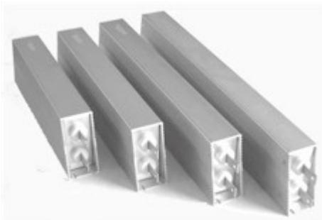
The IRV1600-2800 (V=vertical) models are our highest power, wire wound, metal clad resistors. These models have an extruded aluminium housing providing strong and rugged protection. Options include flying leads or tab terminals and inductive or non-inductive windings. The most common applications for these models are: motor drives, braking and snubber applications and power sources for industrial equipment. These models are fully RoHS compliant.
