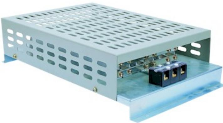
The IRP high power resistor line can handle power of up to 3000W in free air. These models are comprised of multiple resistors housed in a rugged steel protective cover. The base is zinc plated steel. The cover is powder coated which is baked, rendering it extremely strong. The major application for this model range is high power inverter braking resistors.
