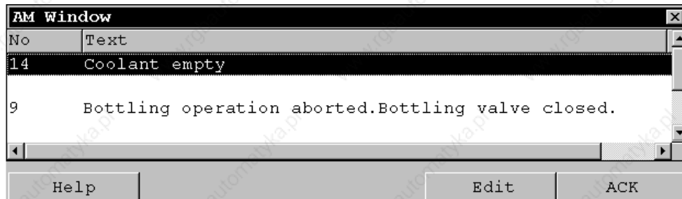
Figure 5-5 Alarm window (example)
