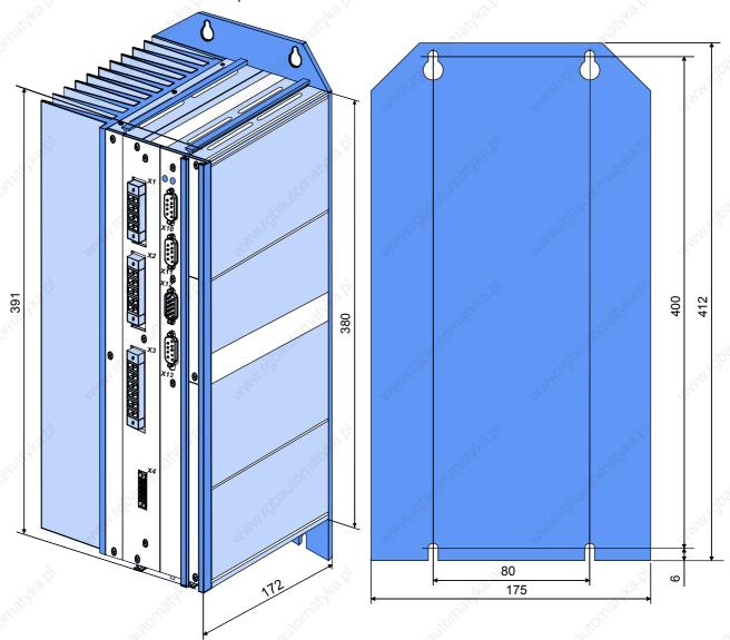
Compax3 S300 V4 is force-ventilated via a fan integrated into the heat dissipater!
