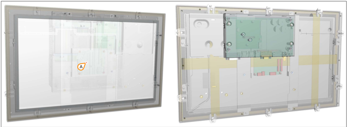
Figure 7: Automation Panel 9x3 - Temperature sensor position
