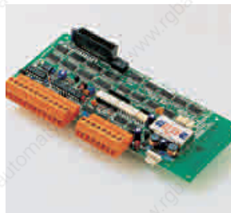
Analogue input board 4 inputs, 10bit resolution
