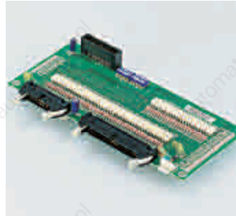
Input board 36 inputs
