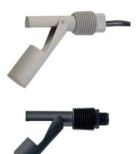
The RSF80 series are designed for mounting through the wall of a tank, via 1/2"NPT thread without requiring acces to the inside of the tank.
