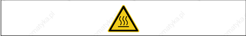
Figure 5: "Hot surface" warning
