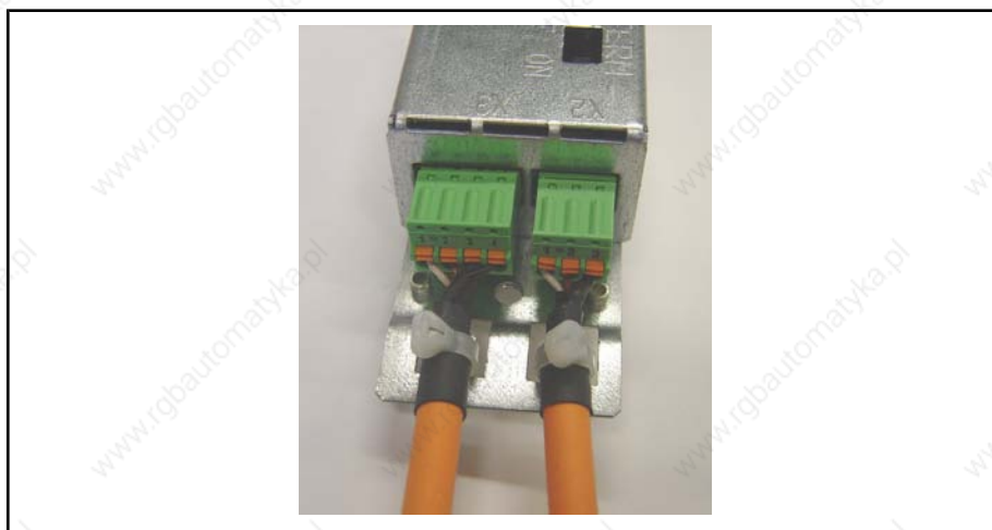
Fig. 14-110: Strain relief at connection X2 and X3
