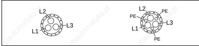
Figure A-2 Recommended motor cables.
