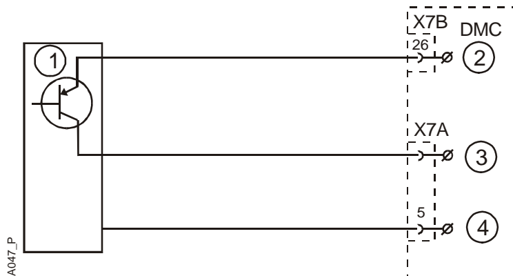
Figure 23. PNP transistor interface to digital input.
