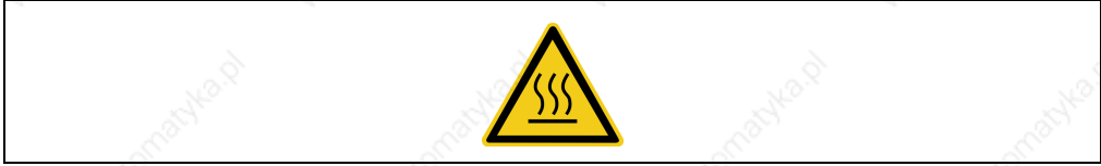
Figure 5: "Hot surface" warning
