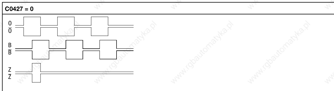
Fig. 3-59 Phase-delayed signal sequence (CW rotation)
