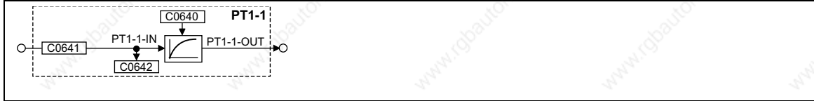
Fig. 3-144 Delay element (PT1-1)
