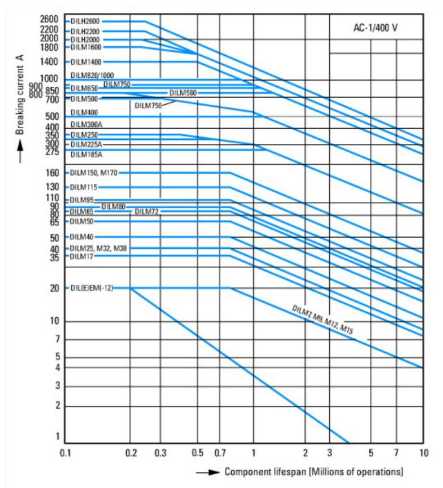
Switching duty for non-motor loads, 3-pole, 4-pole Operating characteristics Non-inductive or slightly inductive loads
