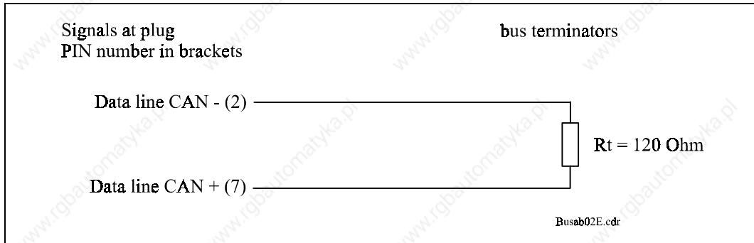
Fig. 48: CAN bus terminators
