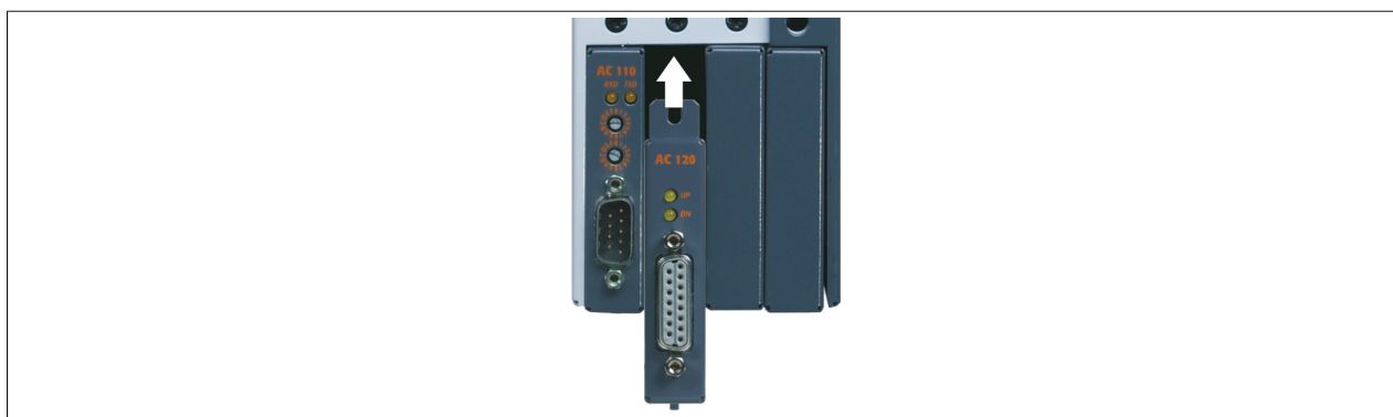
Figure 61: Installing ACOPOS plug-in modules
