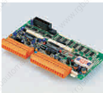
Analogue I/O board 4 inputs/1 output, 8bit resolution
