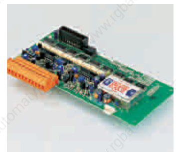
Analogue output board 2 outputs, 10bit resolution
