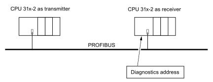
Figure 10-2 PROFIBUS DP diagnostics address
