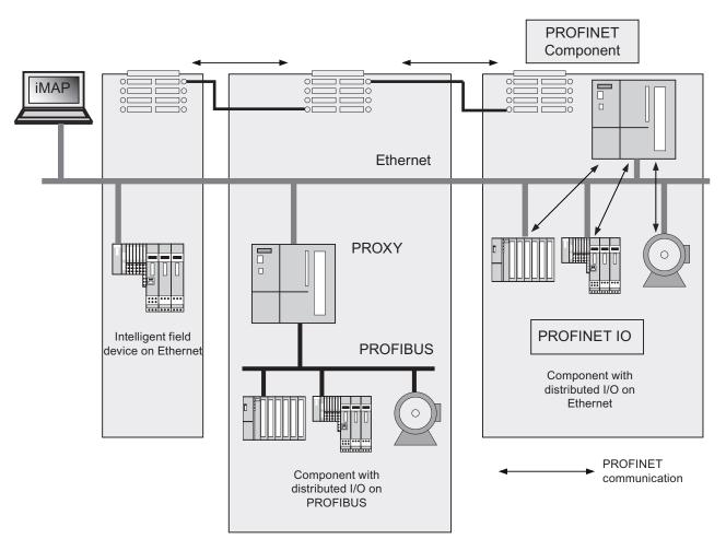
Figure 4-5 PROFINET CBA - modular concept
