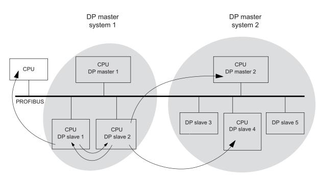
Figure 8-1 Direct data exchange via DP CPUs
