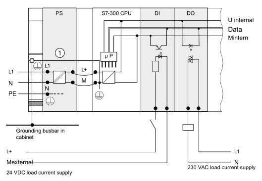
The figure below shows an example of such a configuration: A CPU 31xC with isolated modules. The CPU 31xC (1) is automatically grounded.
