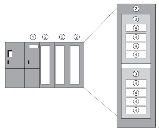
Figure 4-4 Module, Submodule, Slot, and Channel
