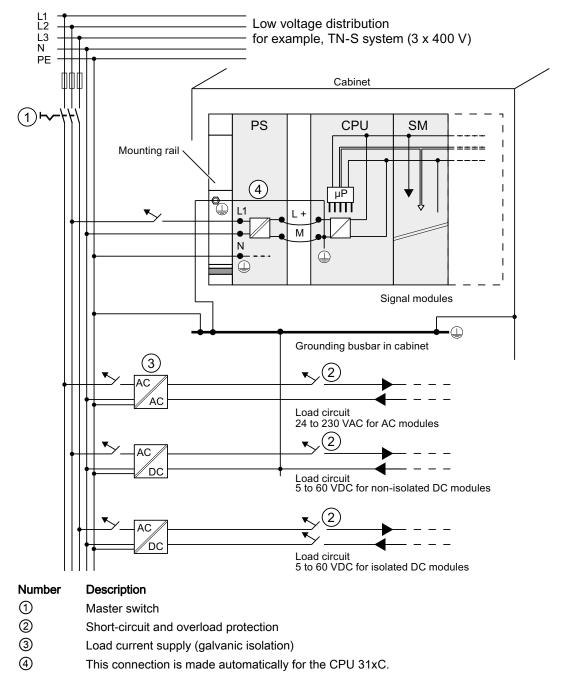
Figure 4-1 Connecting the load voltage reference potential
