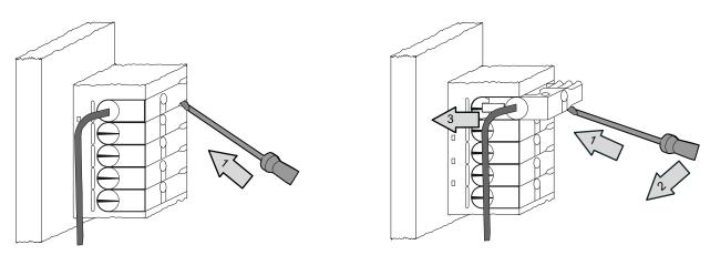
Figure 6-3 Disconnecting the wiring of a 20-pin Fast Connect connector
