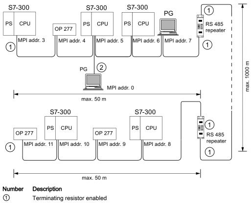
2 PG connected by means of stub cable for maintenance purposes
