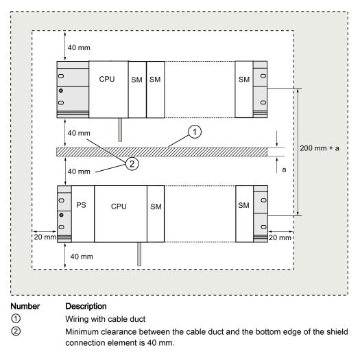
4.5 Arrangement of modules on a single rack
