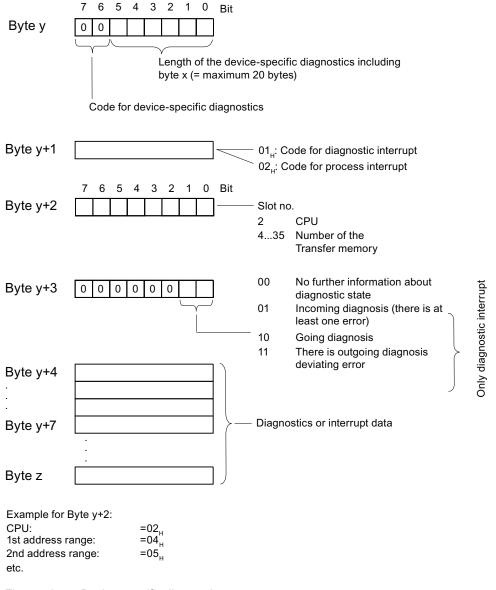
Figure 10-7 Device-specific diagnostics
