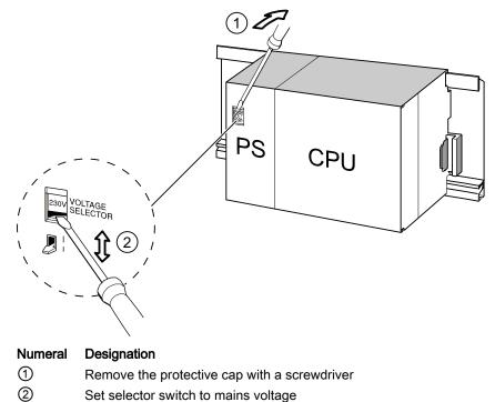
6.4 Wiring the power supply module and the CPU
