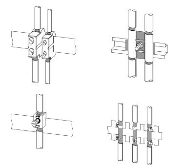
The figure below shows some options for mounting shielded cables, using cable clamps.
