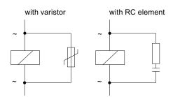
Properties of a protective circuit with varistor:
