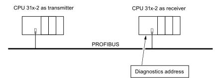
Figure 10-3 PROFIBUS DP diagnostics address
