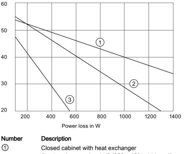
Closed cabinet with heat exchanger (heat exchanger size 11/6 (920 x 460 x 111 mm))
