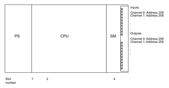
Figure 7-1 I/O addresses of an analog module at slot 4
