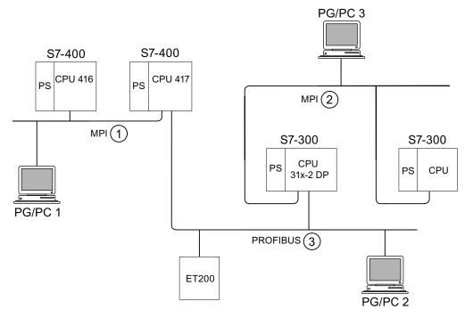
Figure 4-8 Access to remote networks
