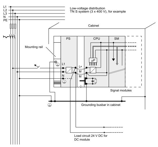
Example: S7-300 with load power supply from PS 307
