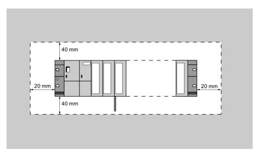
5.3 Installing modules on the mounting rail
