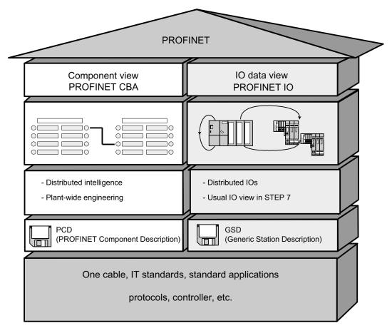
Figure 4-6 Extent of PROFINET CBA and PROFINET IO
