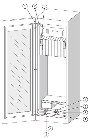
Figure A-1 Example of an EMC compatible cabinet installation
