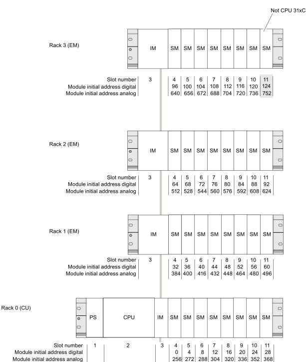
The figure below shows the slots of an S7-300 and the corresponding module start addresses:
