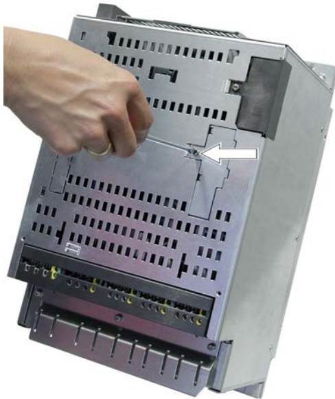
2. Remove the Torx-slotted screw from the fan cover.
