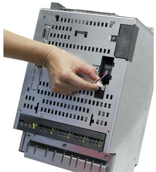
4. Withdraw the connector. To do so, gently press the interlock and connector together.
