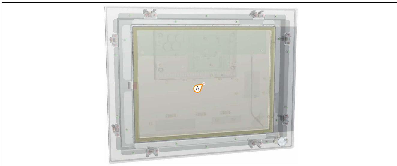
Figure 8: Automation Panel 1000 - Temperature sensor position
