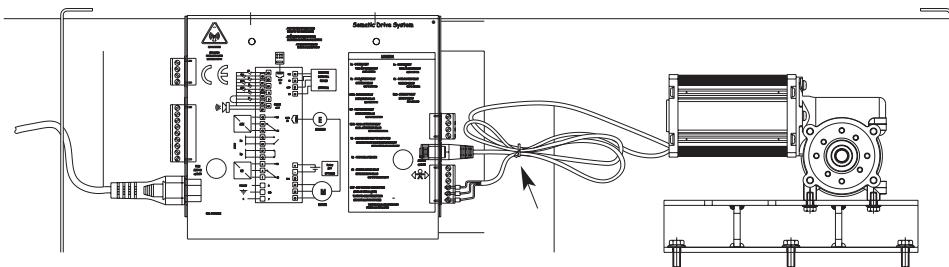
*Note: In case of motor replacement be sure to bind the excess cable lenght as above pictured, to avoid any contact of the motor cable with the driving belt.*
