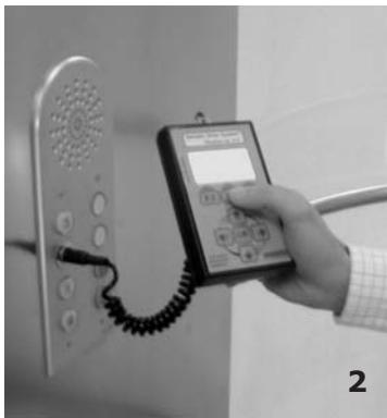
**Note:** when the handset is connected to the controller the display shows the warranty expiration date (2 years from the manufacturer date) and the activity hours left before warranty expiration. Subsequently choose the language by means of the keys **↓** and **↑** and confirm the choice through the "OK" key.
