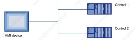
The operator can intervene in the operating process on the HMI device for control purposes. The controller in turn supplies the results of the operating process which are displayed on the HMI device.
