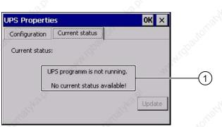
The "UPS program is not running. No current status available." message appears when the UPS is not connected.
