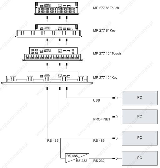
Use a cross-cable for the PROFINET connection when using a point-to-point connection. The interfaces are described in the specifications.
