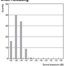
Sample: G5RL-1A-LN 12 VDC Number of relays: 100 pcs Range: A weighted sound pressure level, Fast, Max. hold Device connected to coil: Diode
