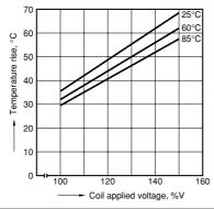
JW 1 Form C High Capacity (10 A) type 1. Maximum operating power
