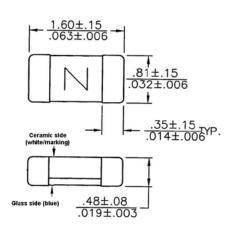
Fuse to be installed with ceramic side up (white/marking)
