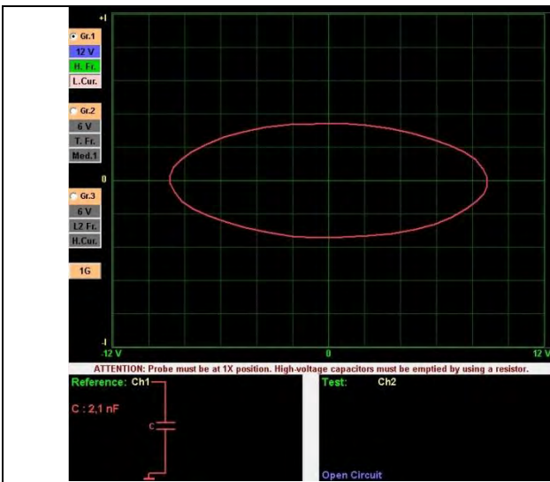
Figure 74: 1.8 nF Capacitor VI Graph
