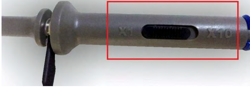
Figure 16: Probe in X1 Position
