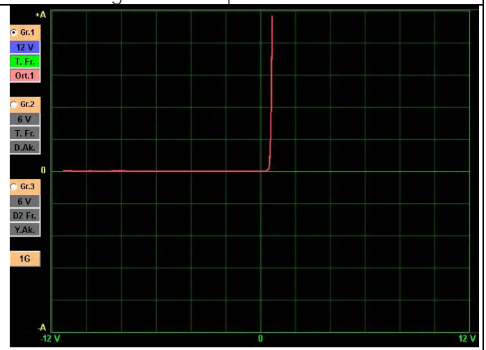
Figure 65: Diode VI Curve
