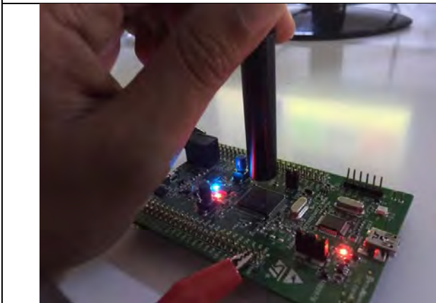
Figure 49: IR Sensor Component Temperature Measurement (Step 7)
