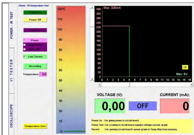
Figure 43: Adjusting the Voltage and Current (Step 1)
