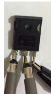
Figure 144: Sample of a Defective N Channel FET
