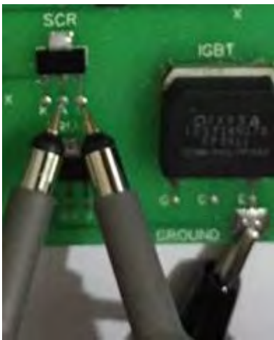
Figure 163: Channel1 (+), Channel2 (+), COM (-) Thyristor Test
