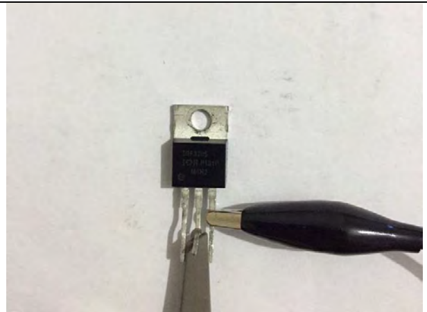
Figure 135: Channel1 Probe Used for Drain - Source Measurement
