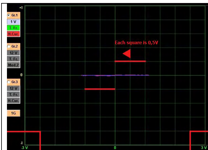
Figure 57: If the Test Voltage 1V, Each Square Represents 0,5V.
