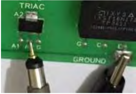
Figure 170: Channel1 Probe Used for Anode2 - Anode1 Measurement
