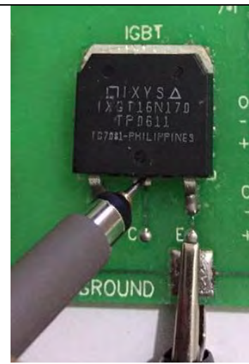
Figure 153: Channel1 Probe Used for Collector - Emitter Measurement
