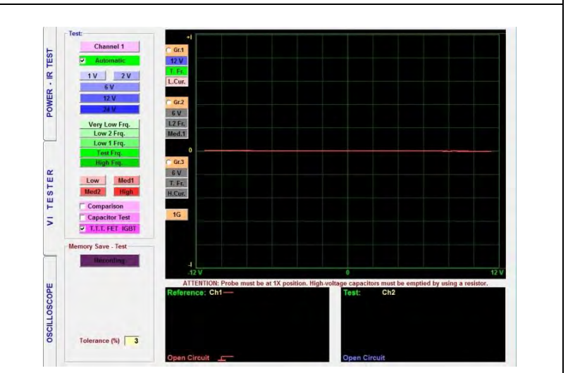
Figure 169: Gate (+) Anode2 (-) VI Graph
