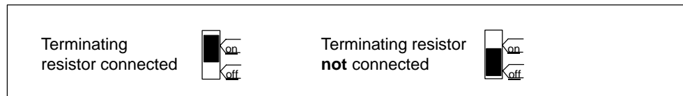
Figure B-1 Bus Connector: Terminating Resistor Connected and Switched Off
