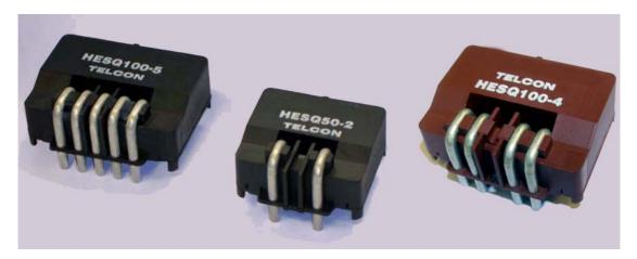
The HESQ 50-2, 100-5 & 100-4 are Hall Element coil and lamination stack assemblies, fitted with isolated primary turns, enabling the implementation of a full Closed Loop Hall Effect Current Transformer by the addition of the requisite electronic circuitry.
