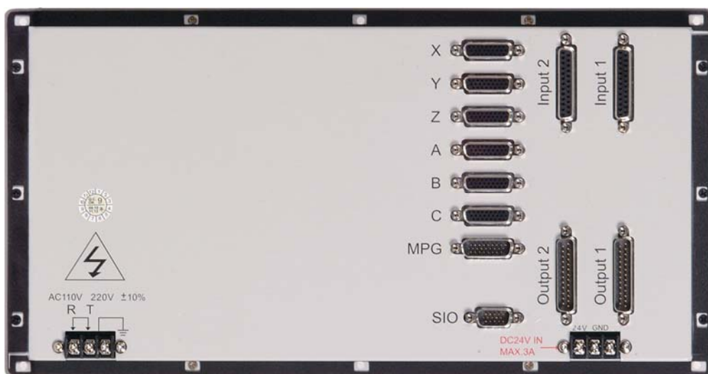
Fig 38 H6D-B CPU Main Board Connectors
