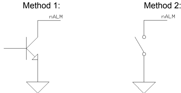
Fig. 2-1-4. Methods of the drive unit providing signals
