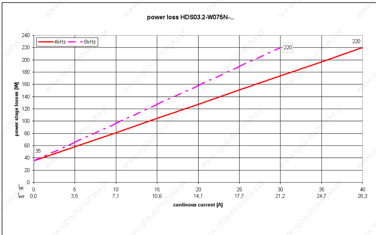
Fig. 7-3: Power loss HDS03.2W075N-
