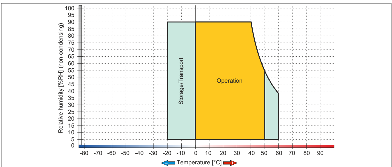
Figure 23: 5AP923.1906-00 ≤Rev. D0 - Temperature/Humidity diagram
