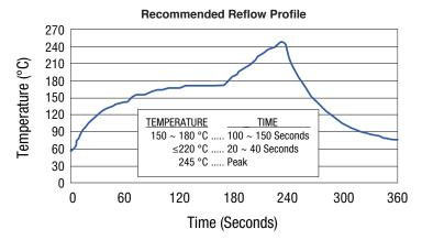
Do not expose the breaker to temperatures exceeding +260 °C.
