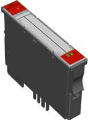
Figure 80: Digitale output module, 2 digital outputs, 24 V DC, 0.5 A, positive switching
