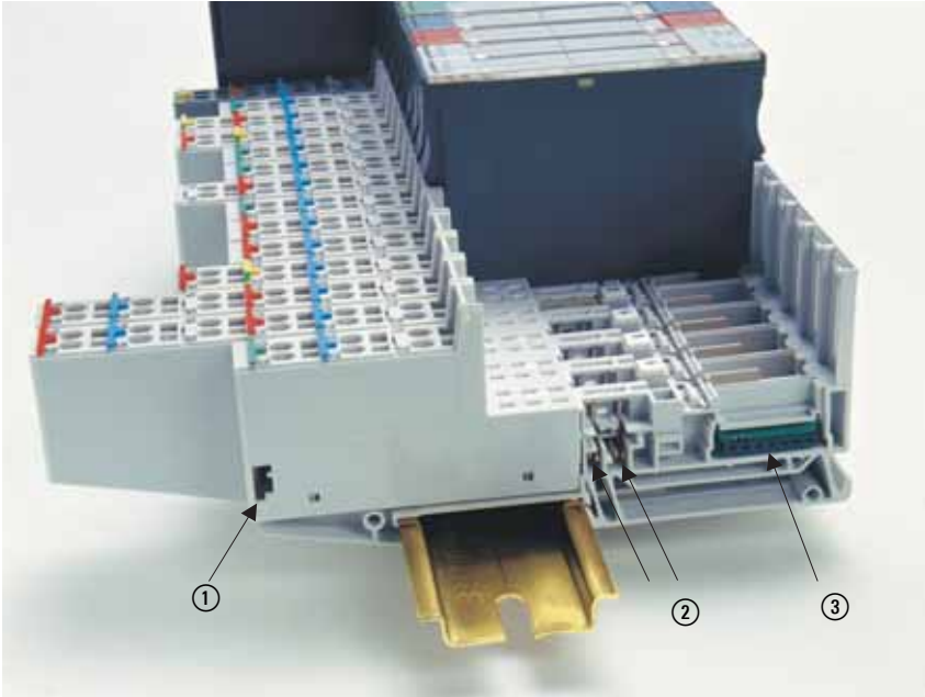
Figure 37: Internal connections in an XI/ON station
