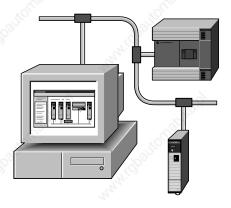
RSNetWorx software is the configuration tool for your control network. With RSNetWorx software you can create a graphical representation of your network configuration and configure the parameters that define your network.
