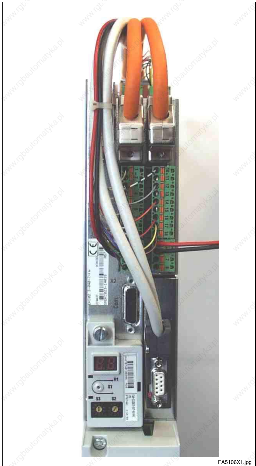
Fig. 16-23: View with Profibus-DP Interface
