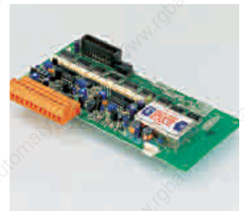
Analogue output board 2 outputs, 10bit resolution
