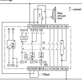
The position of the sliding protective gate is monitored via channel 1 (Y12) and channel 2 (Y22). The SNO 2005-xx is activated through the RESET switch. If the sliding protective gate opens, the E-STOP Relay again drops back into its de-energized state (enable current paths13/14, 23/24, 33/34 open). If the protective gate is closed again, the E-STOP Relay can be activated again through the RESET switch.
