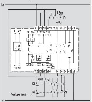
If the number of enabling current paths is not sufficient, two external contactors can be used for expansion. They are driven through one of the enabling current paths of the SNO 2005-xx. The function of the external contactors is monitored through their own normally-closed contacts. The normally-closed contacts are connected in series with the relay K1 (Y13). The contactors K4 and K5 must have positively driven contacts.
