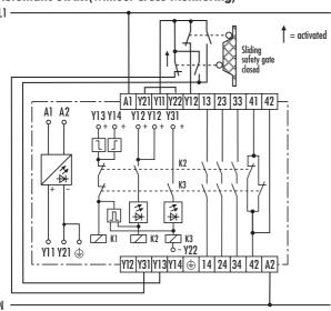
In this application example no simultaneity check ( $t = \infty$ ) is performed.
