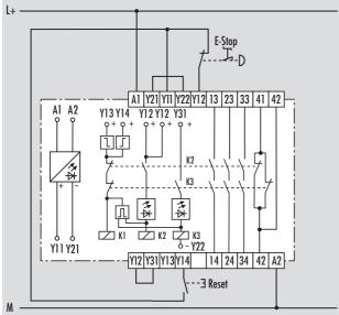
From the relay K3, both actuation connections (Y31, Y22) are conducted to terminals. In this way, the connection to be switched can be chosen at will. The opposite side must be set permanently on plus (Y11) or minus (Y21) by a wire shunt. If the terminal (Y22) is permanently connected to minus (Y21), an E-STOP momentary-contact switch with only one contact can be used.
