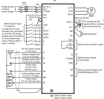
\*\*Connect a single-phase 200V AC input to terminals R/L1 and T/L3(N). \*Factory default settings for relay output are NC contact for AL1 and NO contact for AL2.
