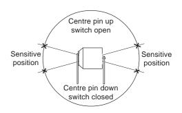
Contact Form/Style: Switch types CM1800 may have a normally open or closed contact depending on the positioning of the switch. These switches have a change in sensitivity depending on the switch position.
