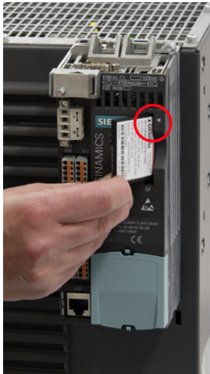
Figure 7-5 CU310-2 PN Inserting the memory card
