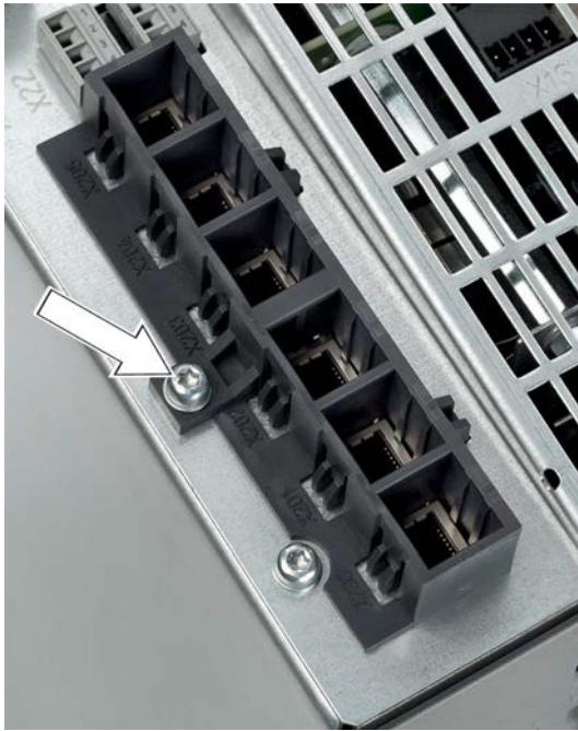
Figure 4-7 Dismantling the guiding frame of the DRIVE-CLiQ interfaces
