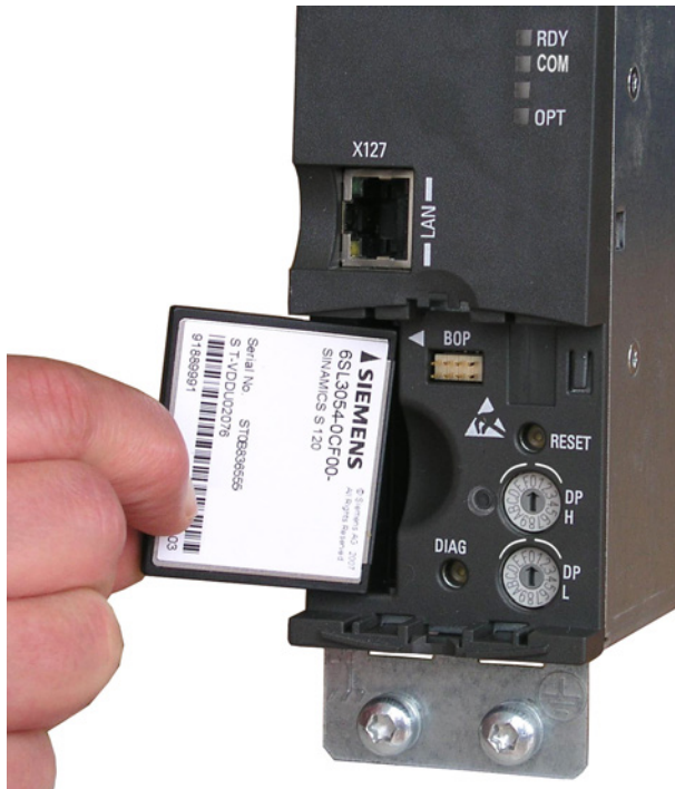
Figure 3-13 Slot for memory card
