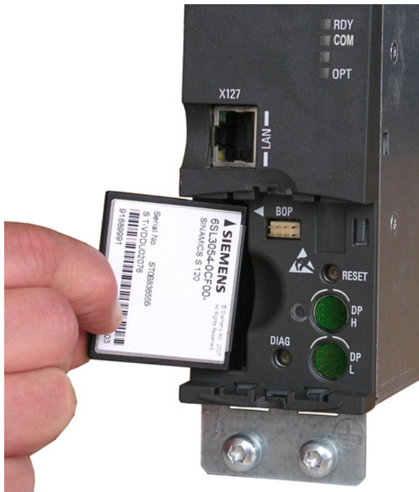
Figure 3-7 Slot for memory card
